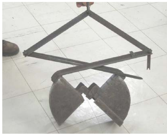
Figure 3-1 Van Veen grabber used for taking the grab samples during the River Survey
